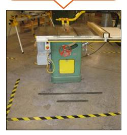
**SOLUTION:** Additional wall outlets may need to be installed to eliminate the need to run cords along the floor. Otherwise, use high-visibility cord covers. Tie up cords that dangle to prevent entanglement.
