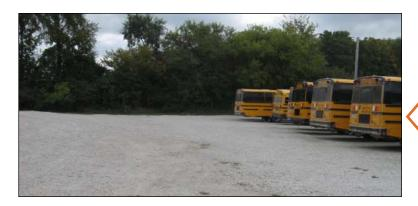
**SOLUTION:** Apply additional gravel to high-traffic areas and areas with thin gravel layers.
